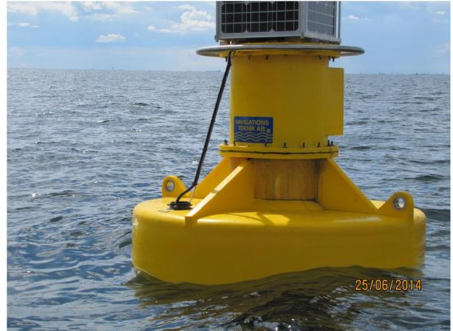
In cooperation with Navigationsteknik, Ocean Origo offers fully equipped data buoys ready for deployment including all necessary components like battery bank, solar panels, nautical equipment, GPS alarm, etc. We also offer complete mooring solutions and mooring components including SeaFlex system for minimizing mechanical mooring stress and customized www-interface. Finally, we also offer installation, service, surveillance and management of buoy systems. In short – we can do it all.
