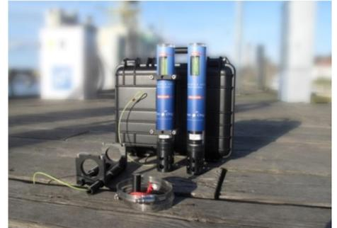
The operator controls SeaTurtle using a small handheld permanent magnet. The instrument can be programmed to enter turn-around mode, string mode, sleep mode, continuously update current temperature/pressure value on the display, show last temperature/pressure registration, etc. SeaTurtle runs on a single ordinary 9 V alkaline or lithium battery cell, easily replaceable by the operator.
