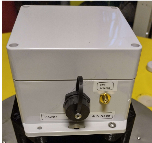
Right: MiniMoose+, here with several SubCon UW connectors. Left: MiniMoose, here with LoRa antenna connector.
